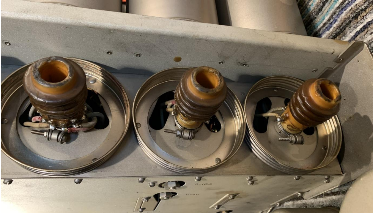
Above: left to right – the TE-236-B detector, 2 nd RF and 1 st RF tuned circuit coils for Bands 4, 5 and 6. Below: left to right - the TE-236-B detector, 2 nd RF and 1 st RF tuned circuit coils for Bands 1, 2 and 3 (these are physically huge for receiver coils!).
