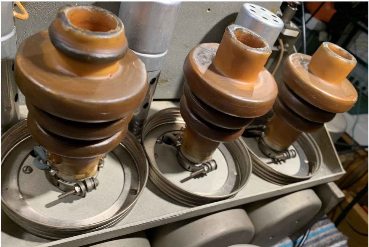
Above: left to right – the TE-236-B detector, 2 nd RF and 1 st RF tuned circuit coils for Bands 4, 5 and 6. Below: left to right - the TE-236-B detector, 2 nd RF and 1 st RF tuned circuit coils for Bands 1, 2 and 3 (these are physically huge for receiver coils!).
